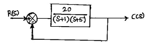
Determine the characteristic equation of the system  $\omega_n$ ,  $\xi$ ,  $\omega_d$ ,  $t_p$ ,  $M_p$  the time at which the first overshoot occurs, the time period of oscillation.
